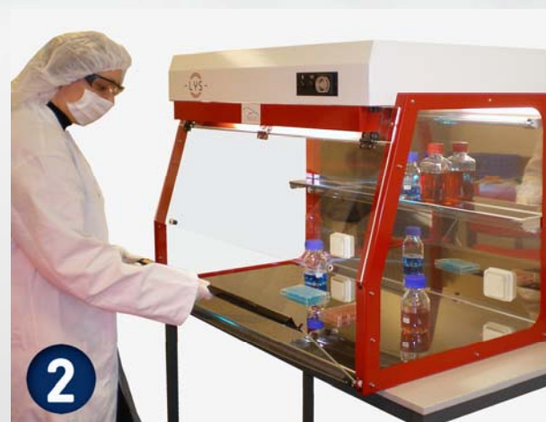
The UV irradiation is automatically switched off when the front window is open.
