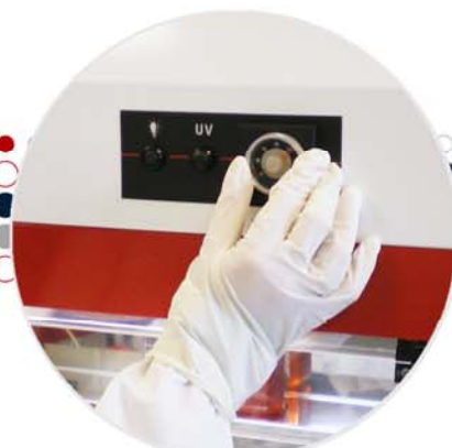
The UV irradiation is automatically switched off when the front window is open.
