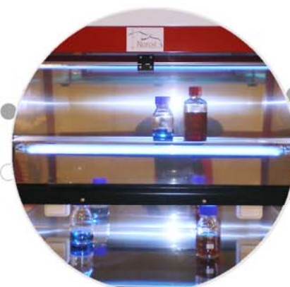
The UV irradiation is automatically switched off when the front window is open.
